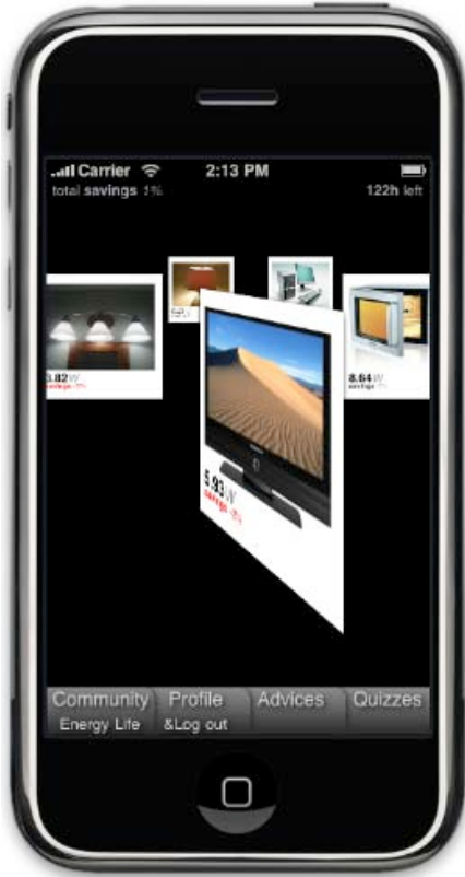
Figure 2. Later prototypes had cards facing the user where the positions of the cards change as the user rotates the carousel. When a card is tapped, it flips around and you can access more content on the backside.
